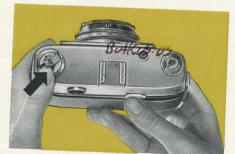
the locking lever to the right (see illustration A on page 2). Then pull out the rewind crank as far as it will go and remove the cassette from the camera, place it in its light-tight packing and mark it as exposed. On operating the rapid transport lever the locking button will spring out again.
